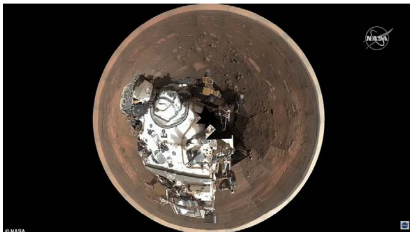
Figure 4. The stunning panorama with 5,000 commands parameters shot a total of 142 images that were directed back to Earth where NASA stitched them together. NASA stitched it together tile by tile in a circular formation, starting with the horizon and ending with the rover
